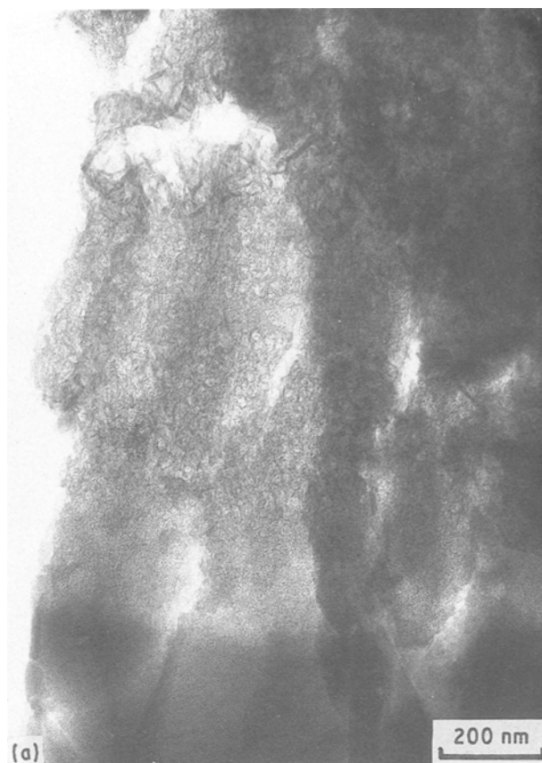
Figure 5 Single filament composite NLP 201-SiC (3 μm thick). Zones 1 and 2. (a) BF, (c) and (d) orthogonal SiO 2 -C 0.2 DF.
